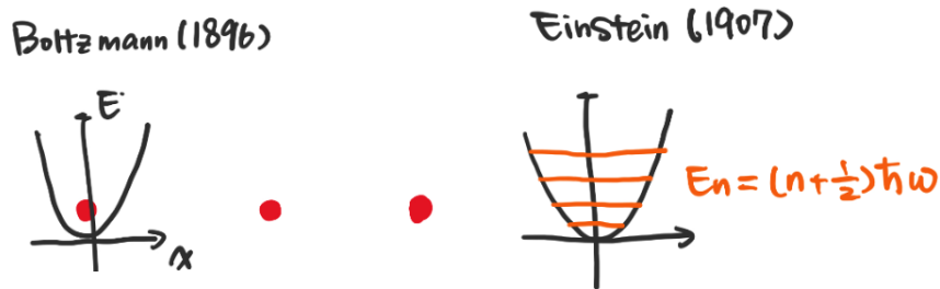
Figure 3: Left: Boltzmann's harmonic oscillator model of atoms; right: Einstein's quantized harmonic oscillator model
